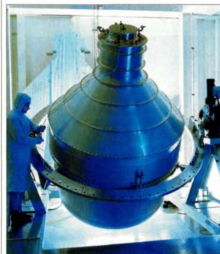
The flight dewar for the Gravity Probe B satellite will maintain the experiment with its four ultra-precise gyroscopes at an operating temperature of 1.8 K.
